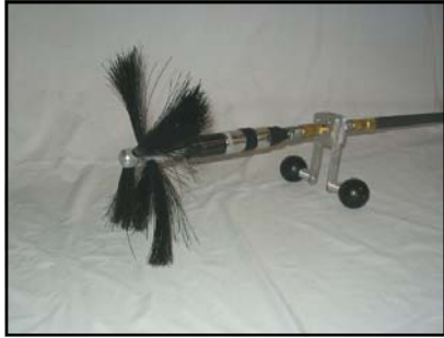
Clean: 4" to 10" ductwork
